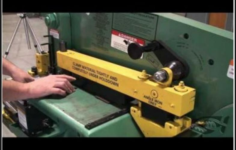
note that the Ironworker is equipped with a small shear blade and typically is capable of shearing plate up to 20-30" in width, Angel Iron, and Barstock.
