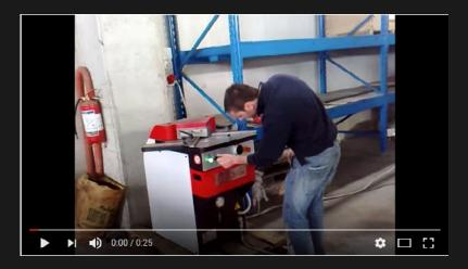
predetrmined angle. Notching only removes metal from the outside of a workpiece. It is capable of making different angle and depth of notches (accomplished by adjusting the location of the workpiece). Notching produces cuts not possible when using the shearing process. To the left is a typical example of a notcher blade assembly.
