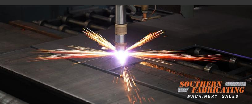
Any kind of thermal processing requires a table to support the material that can withstand the heat and absorb or ventilate the smoke and fumes from the cutting process. In most cases, the table is not part of the initial system quoted and must be calculated for. There are several popular options for tables and they are described as follows:
