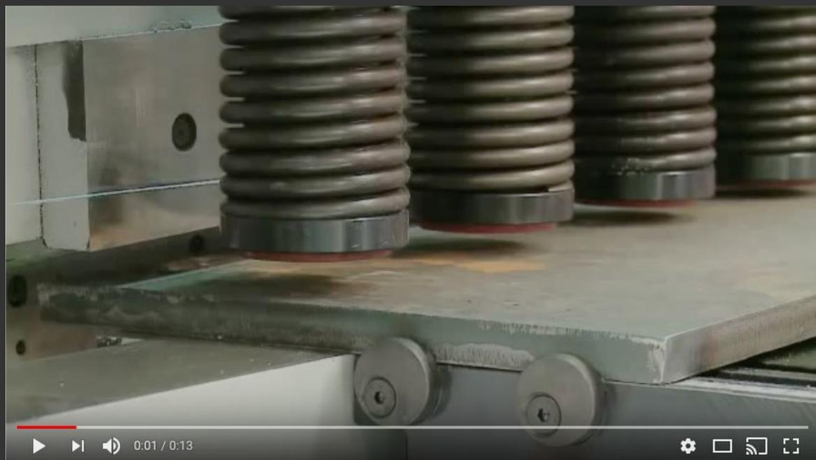
Another shear in action. Note the simple design and lack of a gauging (length measurement) system.
